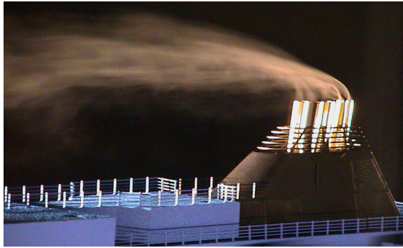
Smoke dispersion test to study funnel performance
