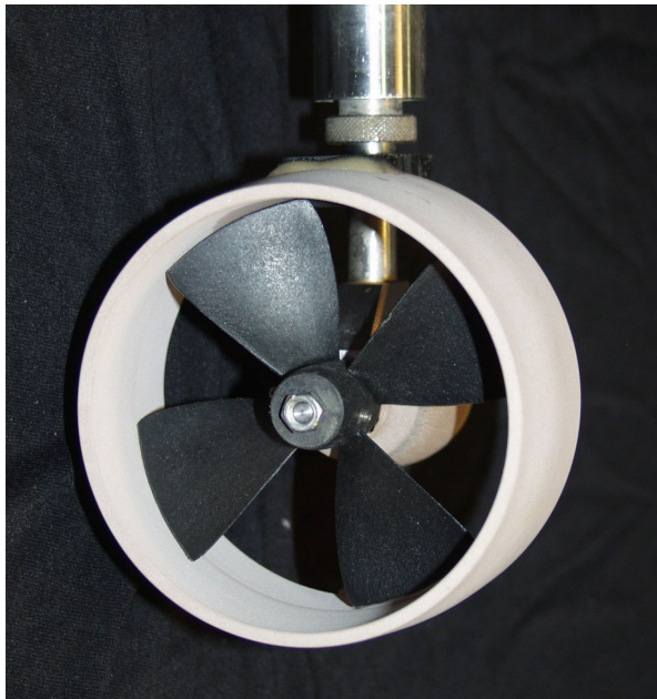
Close-up of offshore thruster unit fitted as azimuthing unit with example of propeller, duct and pod shell
