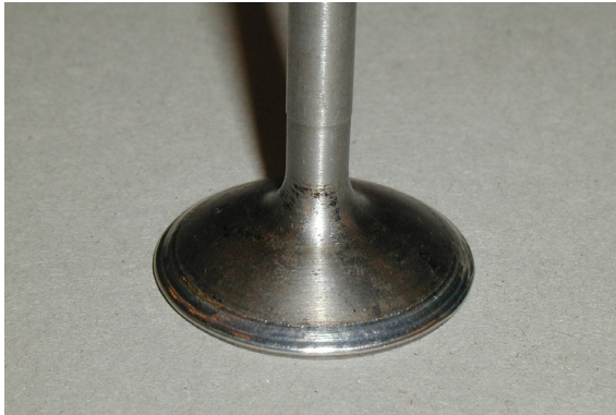
Laser welded valve seat reinforcement
