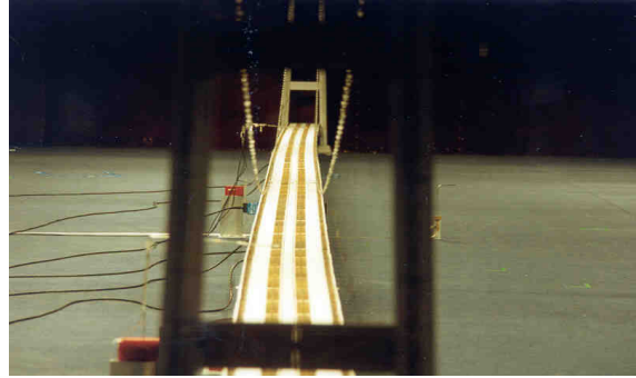
Special equipment tailored for the investigation of the complex response of long-span bridges to the approaching turbulent wind
