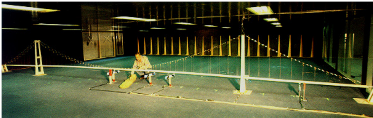
Main purpose of the Wide Boundary-Layer Wind Tunnel is the investigation of the aeroelastic behaviour of long-span bridges under the turbulent atmospheric wind at the location of erection
