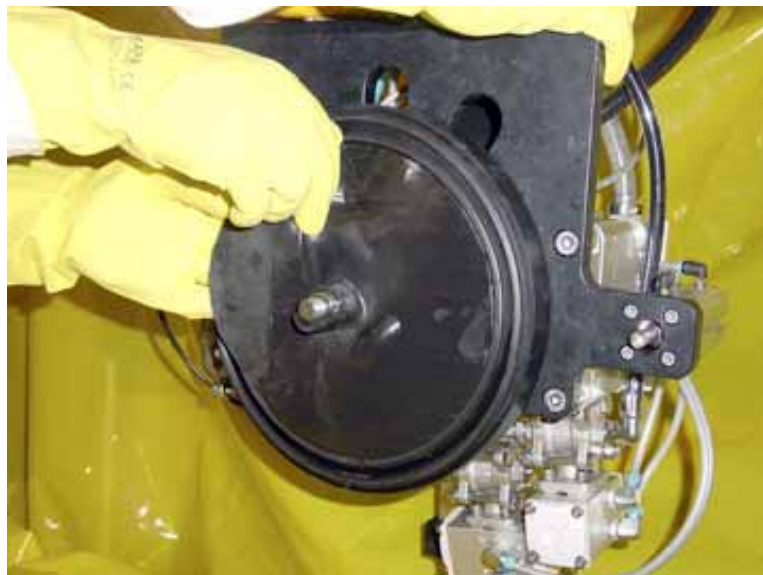
Figure 1. New remote tool for application of moulding material under water. A copy of the level measuring nozzle in the reactor pressure vessel has been made by means of the remote inspection tool.
