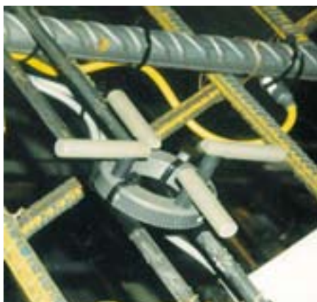
CorroWatch probe and ERE 20 reference electrode
