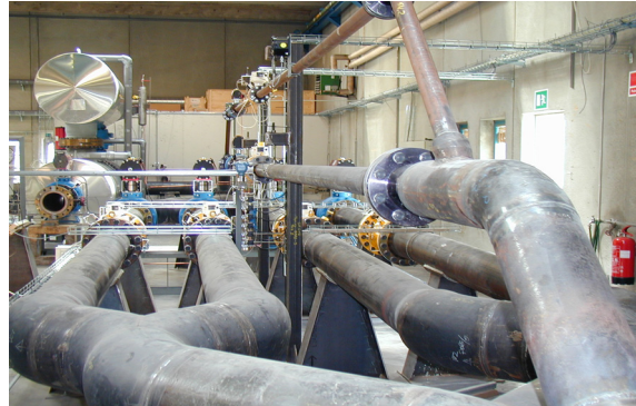
High pressure calibration of volume gas meters and flow meters with natural gas as test medium
