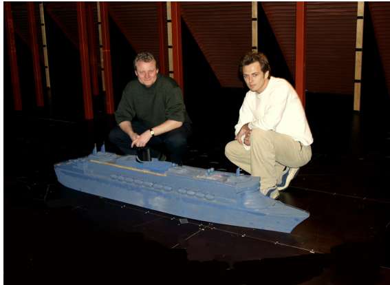
The model of Queen Mary 2 in the wind tunnel
