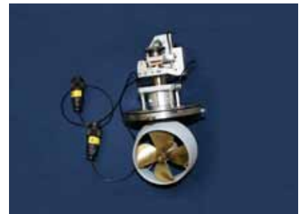
FORCE Technology Mk III offshore thruster model for installation in semi-submersible hulls.
