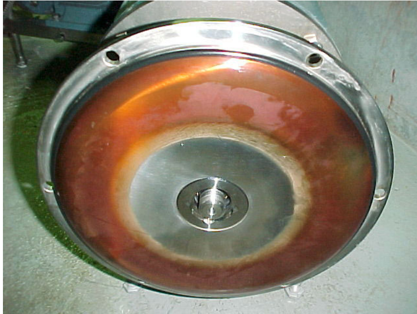
FIGURE 3 - Rouging in a WFI pump.
