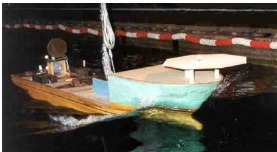
Seakeeping tests in large waves for OSV in FORCE Technology's towing tank
