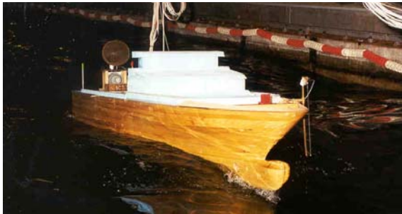
Seakeeping tests for a large luxury yacht in FORCE Technology's towing tank
