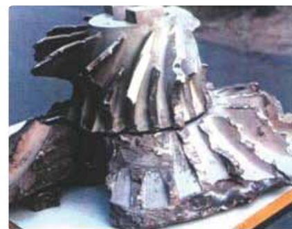
Totally destroyed compressor wheel
