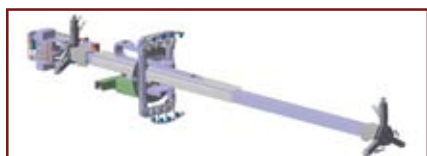
AMS-33 with probe holding system, rotation drive and longitudinal rail drive
