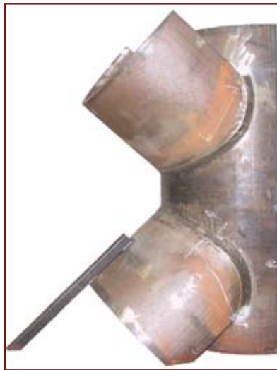
1830 mm high mock-up of platform leg with brace welds. The wall thickness of the leg is 45 mm and its internal diameter is 940 mm.
