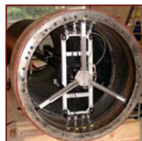
AMS-33 installed for scanning
