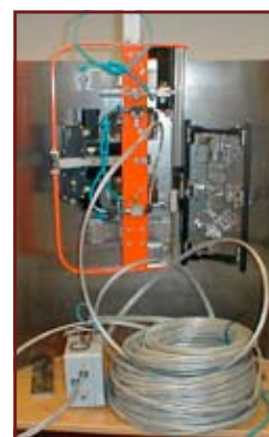
The AWS-5D scanner equipped with 4 magnetic wheels, 2 motors and 7 UT probes mounted on the Y-drive arm. The scanner is fitted with 4 pneumatic operated guide wheels for release of the magnetic wheels.
