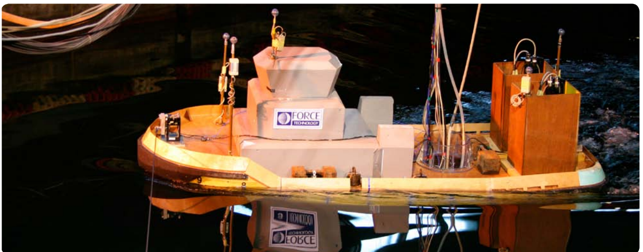
Escort test with ASD tug in FORCE Technology's towing tank
