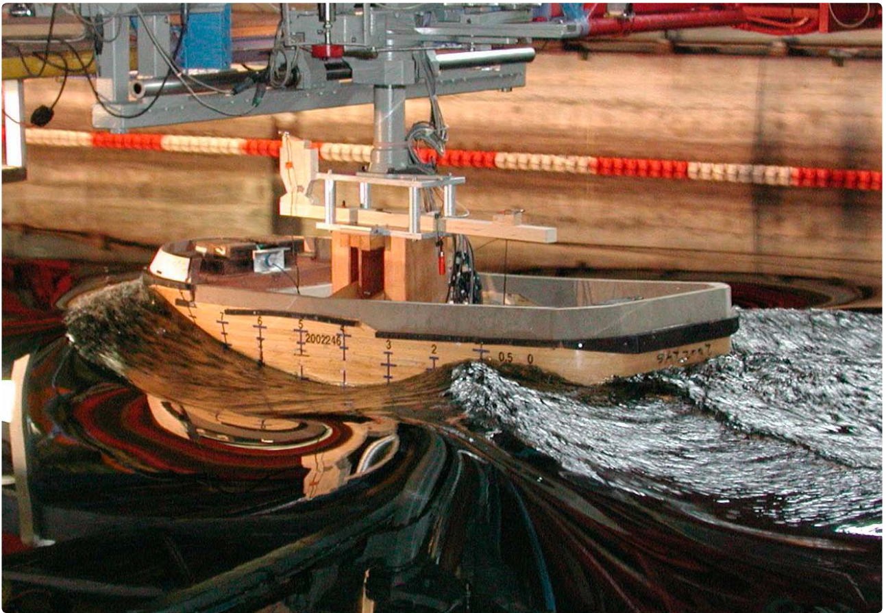
PMM test with ASD tug in FORCE Technology's towing tank
