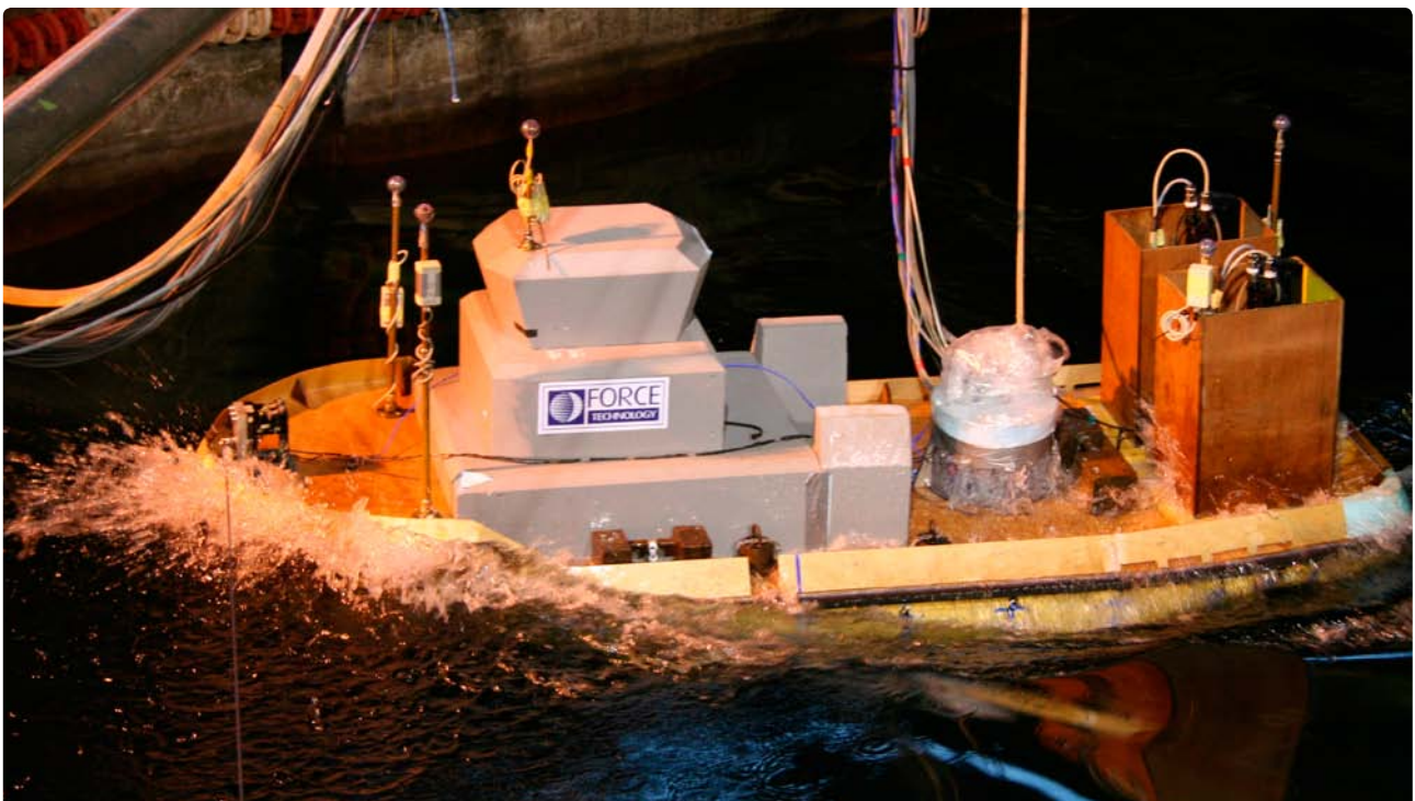
Escort test with ASD tug in waves in FORCE Technology's towing tank.
