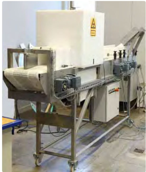
Photo: The NiCd-sorter demonstration device is mobile, enabling demonstrations performed on site
