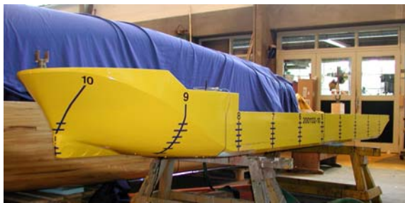
Model Turbine Installation Vessel ready for tests
