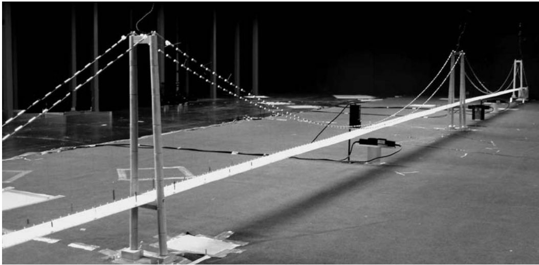
Figure 3. Photograph of the aeroelastic model in FORCE Technology's 13.6 m wide wind tunnel.
