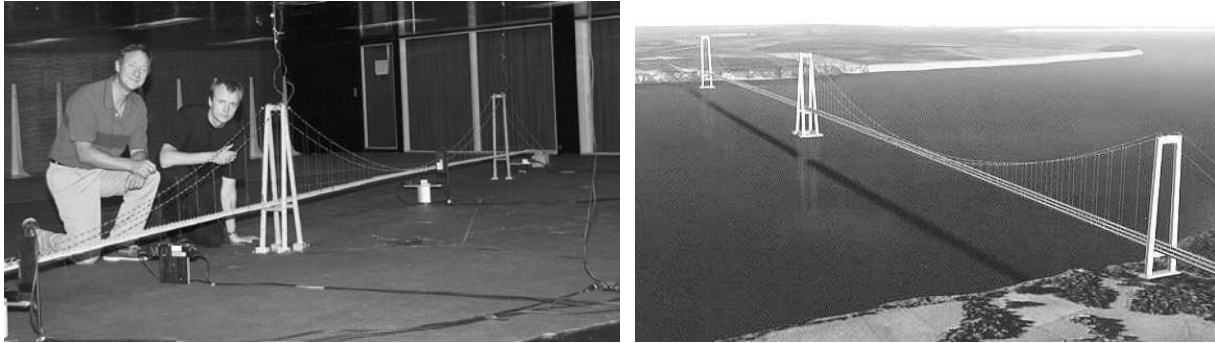
Figure 5. a) Photograph of the 1:215-scale full-bridge model at 30° yaw angle with the authors and b) graphical illustration of the full-scale structure.
