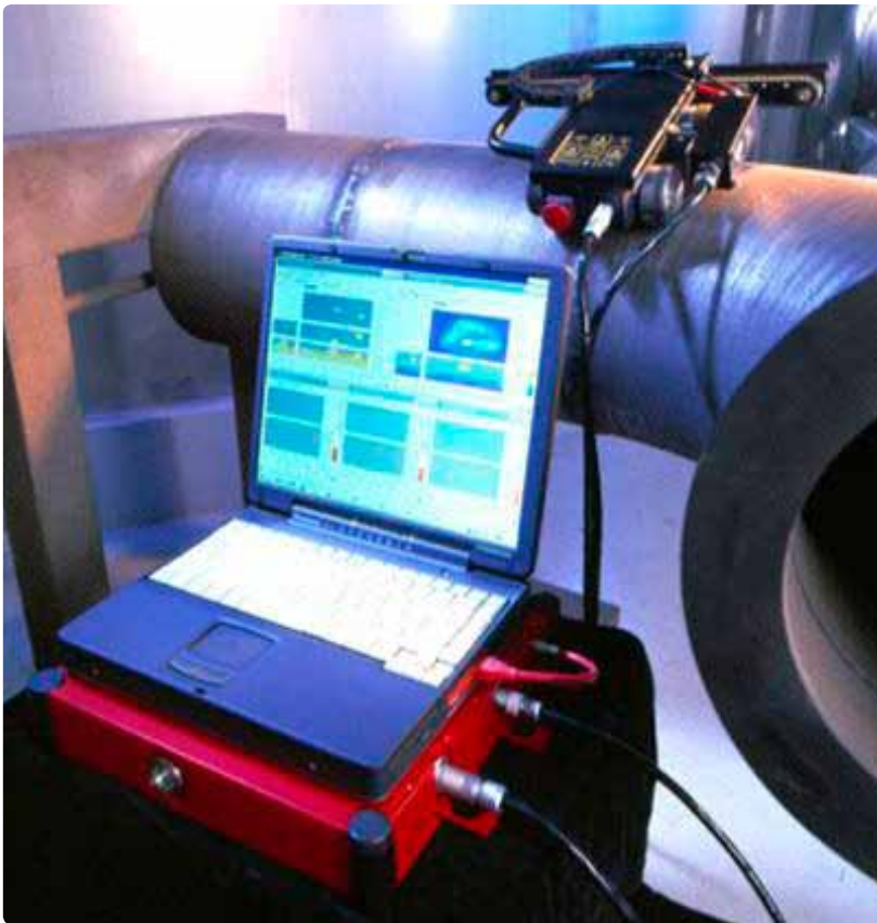
P-scan 4 Lite: PSP-4L with Industrial Notebook PC and AUS-3 scanner
