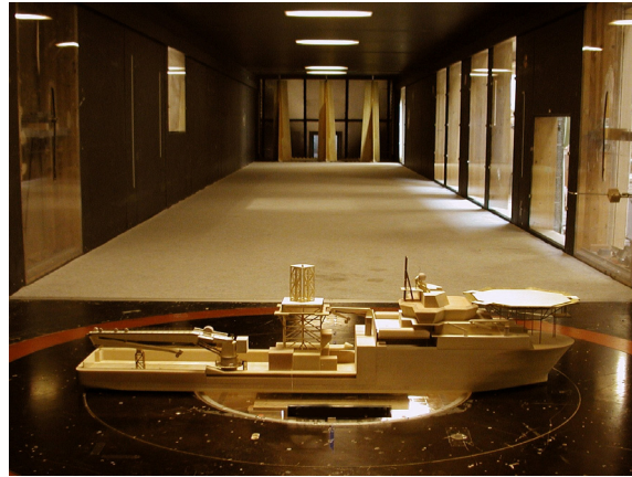
The above-water part of a vessel in the wind tunnel
