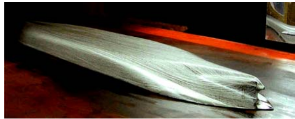
Streamline test in the windtunnel on model of an AFRAMAX Tanker.
