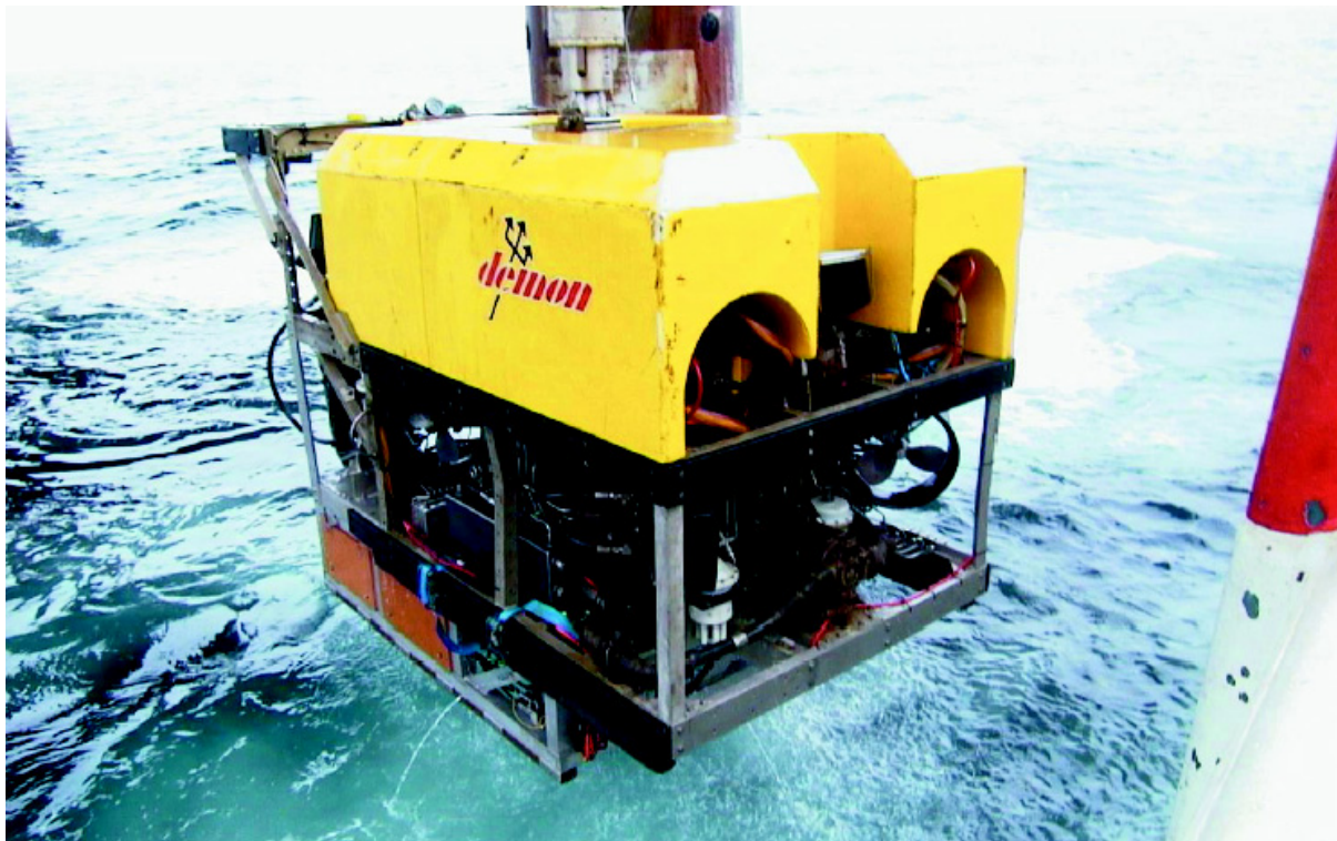
ROV with P-scan 4 and AUS-4 subsea scanner mounted on tool skid
