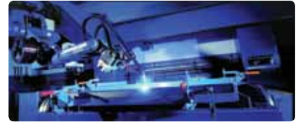
FORCE Technology is involved in an ATF project which is studying the possibilities of using powerful fibre lasers for joining heavier material thicknesses such as in offshore wind turbine foundations and wind turbine towers.
