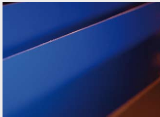
A few panels ready to be tested. The panels were ordinary metal plates prepared with undercoatings emulating real life surfaces before being coated.
