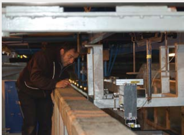
The testing rig was developed with particular focus on simple but high mechanical accuracy and the capacity to test many panels with different types of fouling control coatings.
