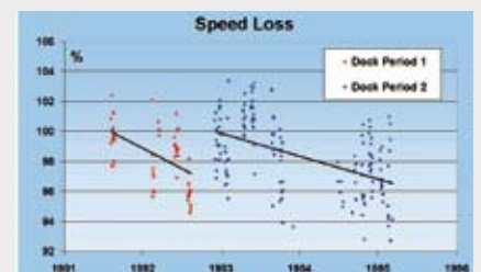
Significant speed loss as a result of fouling. ■
