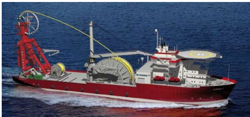
Subsea 7 Seven Oceans - Deepwater rigid pipelay vessel built at Merwede Shipyard.
