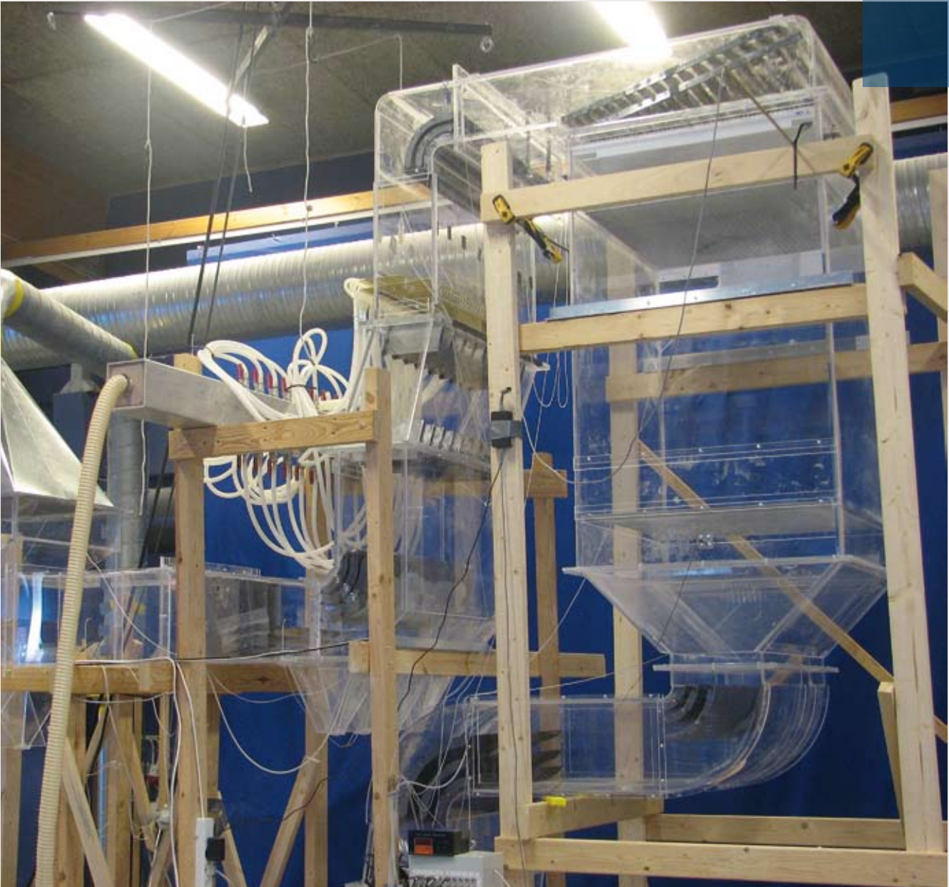
Scale flow model, dimensions 1.8 x 4.2 x 4.6 meters, excluding adjacent equipment.
