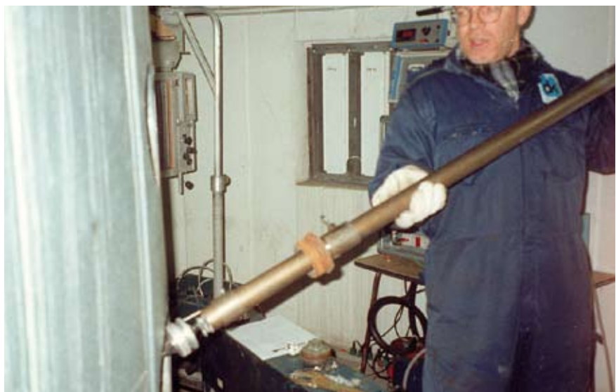
Manual measurements of particulate emissions are often carried out in stacks/chimneys, with limited space to handle the needed 2-4m long probes.
