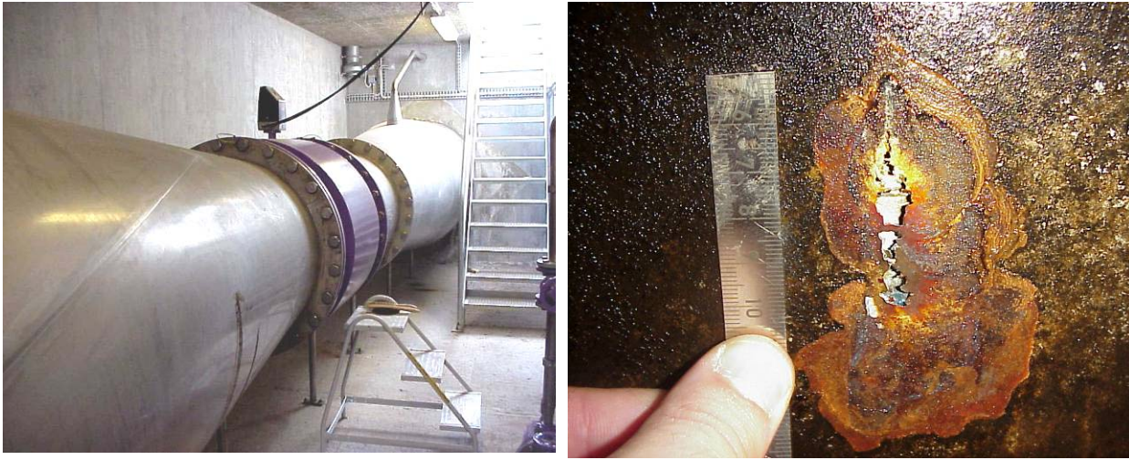
FIGURE 2 - Pits in AISI 304 base material at the outlet flow meter in sewage treatment plant H. a) overview showing two penetrations, b) extensive attack surrounded by \text{MnO}_2 deposits on the inside.
