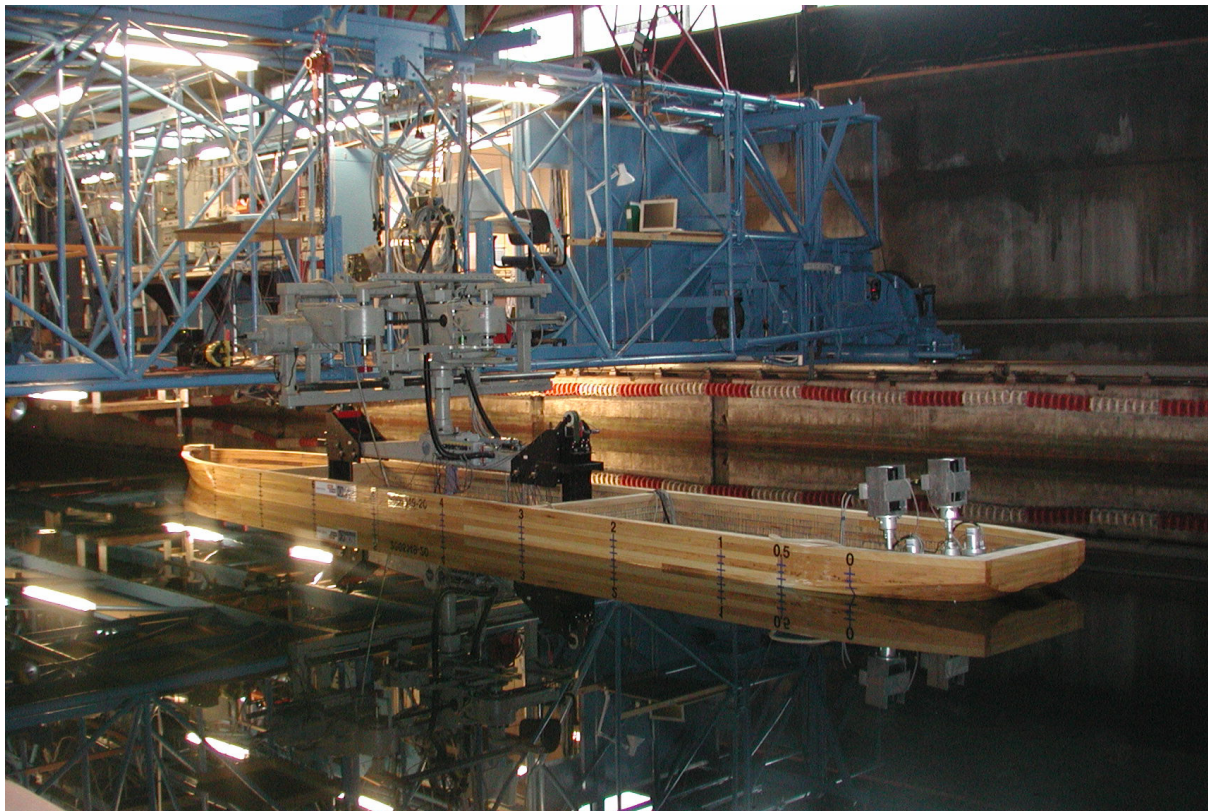
PMM Manoeuvring tests in the deep water towing tank
