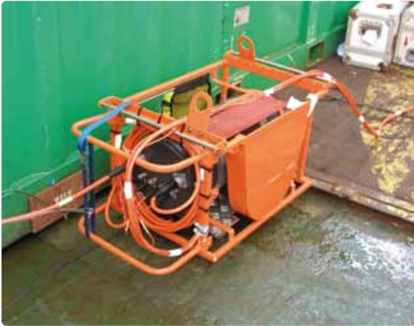
Photo: P-scan diver skid.
