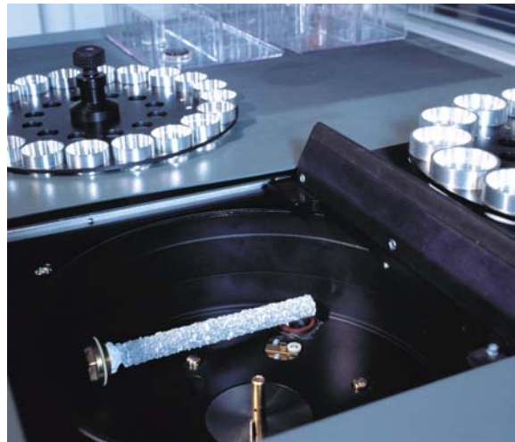
An anode with coating in the test chamber
