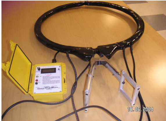
DC clamps for CP current readings in pipes, mooring chains etc Permanent and ROV operated.
